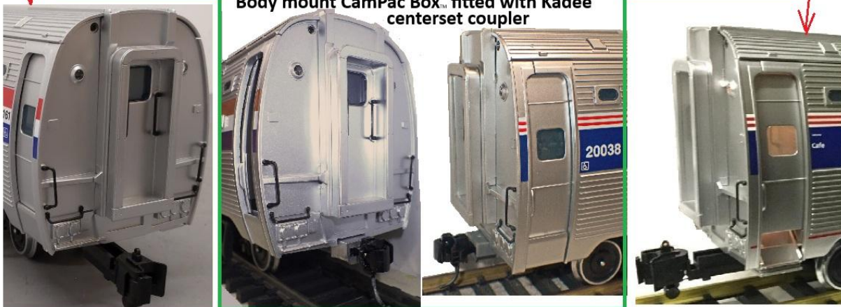
CamPac box coupler alignment with Kadee 980 coupler height gauge
