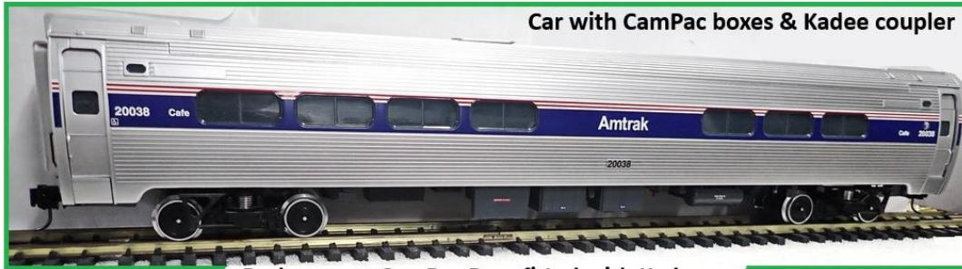
Body mount CamPac Box™ fitted with Kadee centerset coupler
