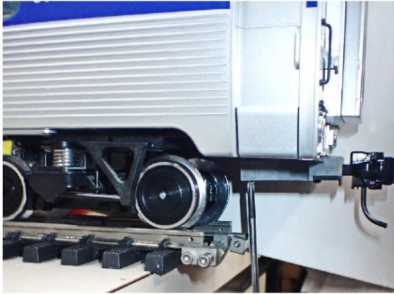
Place Amfleet car on straight track on a table with one end over hanging
