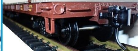
Car with body mount CamPac Boxes™ fitted with Kadee center set couplers from 907 kit and USA Trains metal wheels
