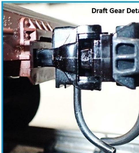
Coupler Alignment with Kadee 980 gage
