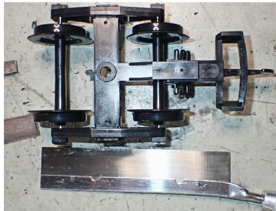
Example Razor Saw used to cut off tang
