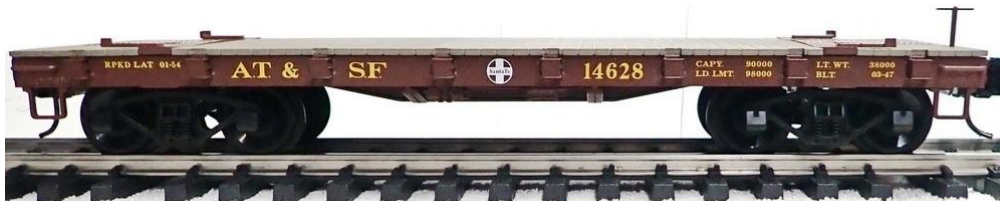
Car with body mount CamPac Boxes™ fitted with Kadee center set couplers from 907 kit and USA Trains metal wheels
