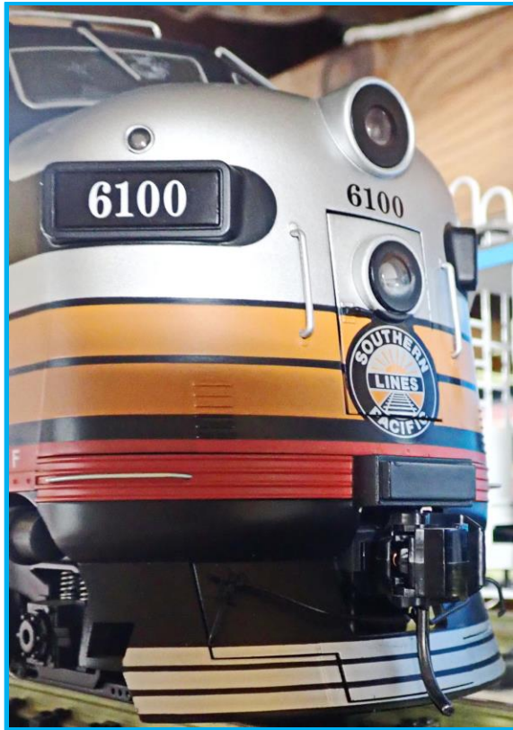
Example USA Trains F3A with CamPac Box™ and centerset coupler coupled to USA Trains Streamliner car fitted with body mount center set coupler
