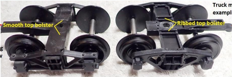
Place large 0.050 inch thick truck spacer washer over frame bolster post
