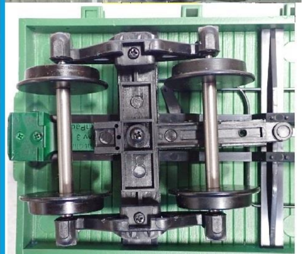
Remove couplers from truck tangs and plastic (or under/over sized aftermarket wheels compared to USA Trains metal wheels). Replace with USAT metal wheels, PN R2093
