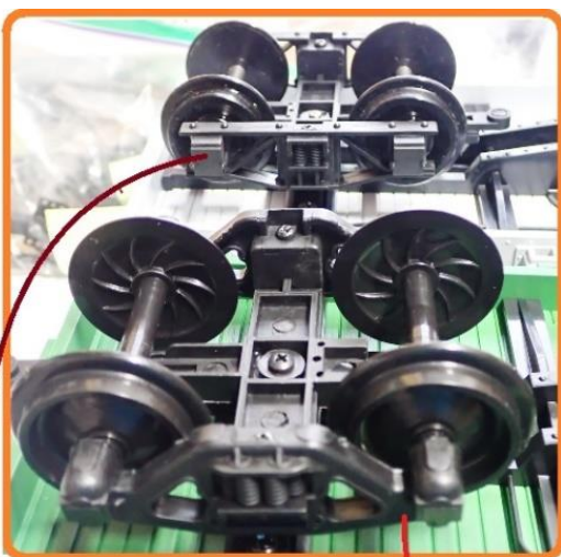
Both example cars have trucks with ribbed top bolsters
