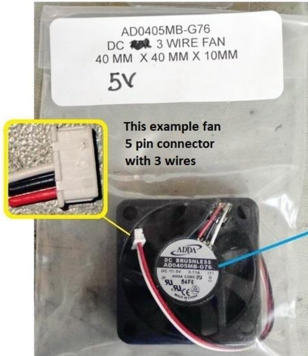
Only red (+) and black (-) wires used for powering fan
