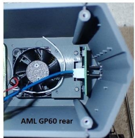
Only red (+) and black (-) wires used for powering fan
