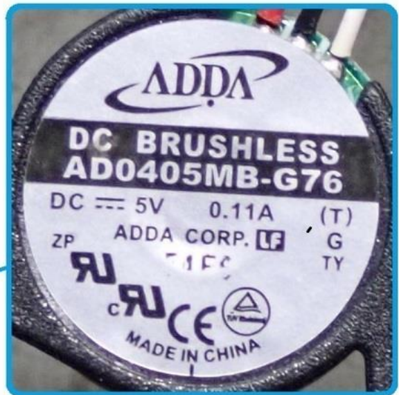
Only red (+) and black (-) wires used for powering fan
