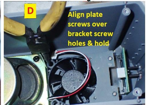
Alternately thread-in mounting screws until fully seated
