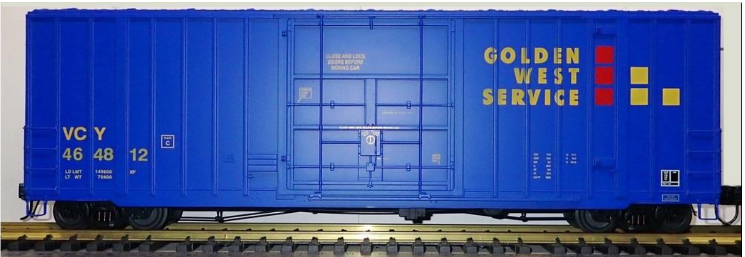
Example AML Hi-Cube 50 foot boxcar equipped with CamPac Boxes™ fitted with Kadee* centerset couplers from 907 kit
