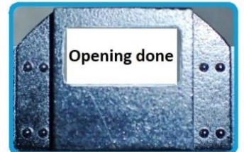
Using various files, enlarge draft gear opening until lines just disappear with corners squared-up
