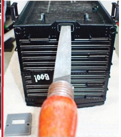
Using various files, enlarge draft gear opening until lines just disappear with corners squared-up
