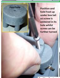
hold Foot up under box tail so screw is centered in its hole whilst screw can be further turned
