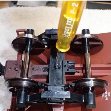
With coupler tangs having been removed, re-mount trucks using factory washer & screw.
