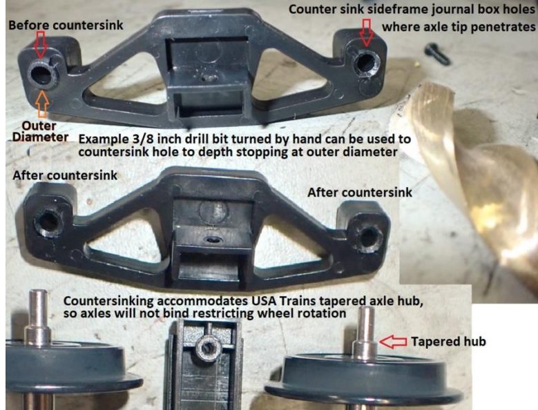
Install USAT metal wheels
