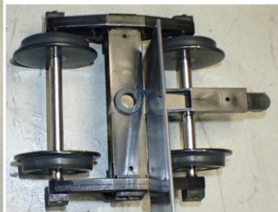
Factory Trucks must have their coupler tang removed when using body mount couplers - Example shown with wheels in place using razor saw
