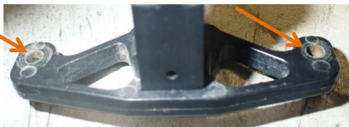
Factory Trucks must have their coupler tang removed when using body mount couplers - Example shown with wheels in place using razor saw
