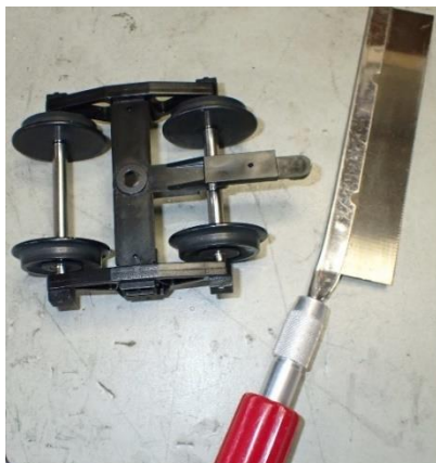
Factory Trucks must have their coupler tang removed when using body mount couplers - Example shown with wheels in place using razor saw
