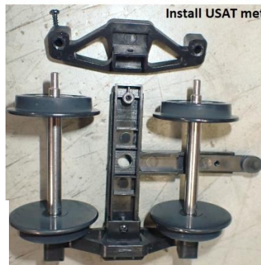
Install USAT metal wheels
