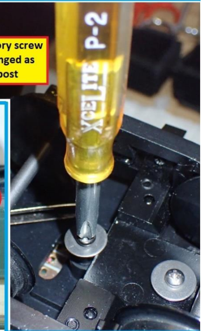
When inboard axle of truck is pressed down, truck will be vertically limited, so when truck rotated, it will be very close to chassis boss
