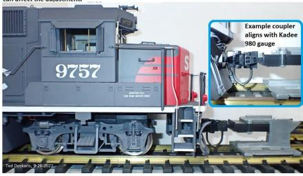
Illustrated is a variety of possible AML GP60 lash-ups given the projection of the CamPac coupler boxes fitted with Kadee centerset couplers to like kind Kadee equipped items.
