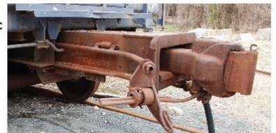
Example Prototype Cushion Capable Coupler Draft Gear Box with characteristic pronounced projection from end of car
