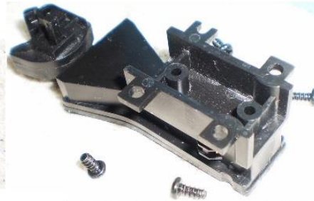
USA Trains Cushion Coupler Assembly with factory Spacer
