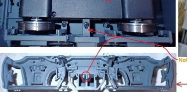
indicative of camber angle of installed sideframe, therefore, adjustable to be parallel to side of motor block Interior of sideframe shown after it's withdrawn from the truck's motor block Ted Doskaris, 10-4-2021
