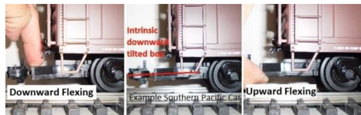
The USA Trains 60 ft boxcar chassis where the coupler box is mounted is predisposed with a downward tilt and is too flexible. This is corrected when mounting the CamPac box™ with added end bulkhead screw.
