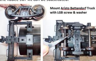
Mount Kadee 70 & 100 ton "Roller Bearing" Trucks same with only Adapter kit's LGB short length "Hat" 🔒 Hat and LGB screw only - no washer
