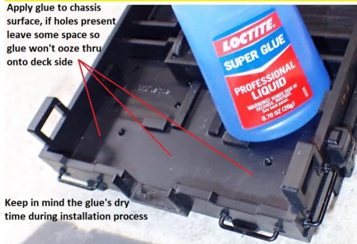
Trial fit CamPac Plate before gluing to ensure it seats perfectly flat
