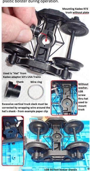
With trucks installed, car coupler alignment with the Kadee 980 gauge will likely require shimming the CamPac Box – described in sheet 7. See illustrated descriptions below when **Choosing the Aristi-Craft Barber ART-29100** roller bearing truck.
