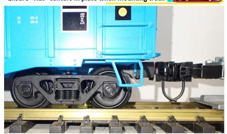
**Method 2, shown below**, optimally lowers the car, but it may result in greater wear of the car's plastic bolster during operation.
