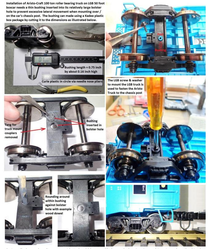
With trucks installed, coupler alignment with Kadee 980 gauge likely needs CamPac Box™ shimming - described in sheet 7
