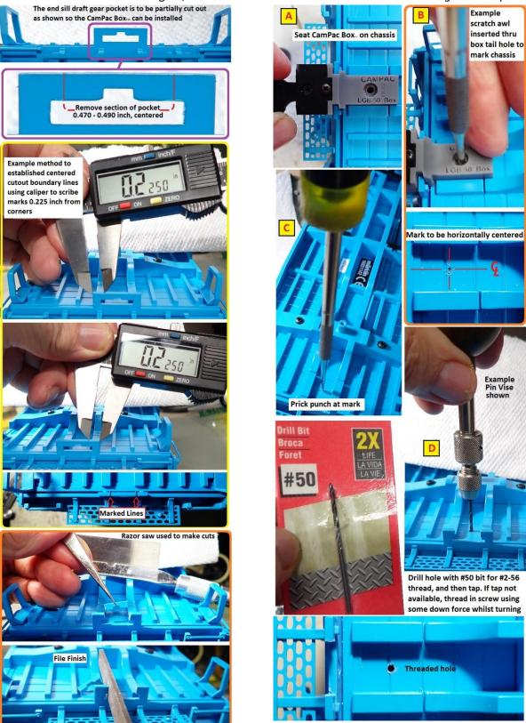
A #2-56 by ½ inch screw is used to fasten box to chassis.
