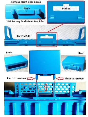
Modifications to car: First the draft gear, and then drill hole to mount CamPac Box™ - using it as template
