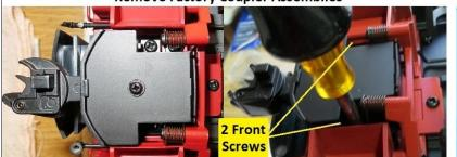
To remove screws at bracket feet, a narrow shank Phillips screwdriver is needed with it being held at an angle for screws under the springs
