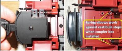
Remove Factory Box from Bracket (Bracket will be used with CamPac Box) Remove small center screw that retains lid to box, and then pry away back of lid to disengage tab from rear slot to remove it, and then withdraw the coupler and its spring from the box. (Spring may separate & fly out!)
