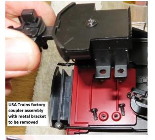
CamPac Box<sup>TM</sup> fitted with Kadee centerset coupler to be inserted within factory metal bracket.
