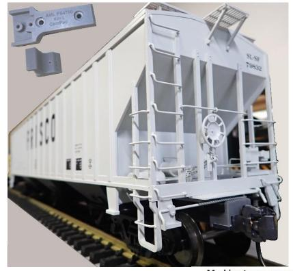
Trucks are to be temporarily removed and then have their factory coupler tang removed. This is required for rotational clearance once trucks are reinstalled following the installation of CamPac parts.
