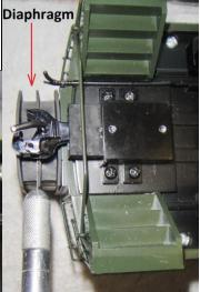
**Note:** Because the Kadee coupler does not pull out like the USA Trains spring loaded coupler; car spacing is not affected during operation of the car in a train. **Shown below CamPac Box/pedestal is installed for coupler projection like factory**
