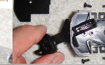
Remove the 2 metric M2.5 by 8mm flathead screws that fasten the box to the pedestal. Keep these screws to install the CamPac Box.
