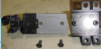
The CamPac Box is installed within the pedestal using the factory M2.5 by 8mm flathead machine screws. Installation can be done two ways: The first shown below at the far left is to be like the factory coupler projection at the diaphragm end, whereas, the second shown at the middle is to be recessed for closer car coupling. In this case, the diaphragm shown at the far right would have to be shortened by one flute, or it could be removed.
