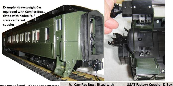
CamPac Boxes fitted with Kadee\* centerset knuckle coupler from the 907 kit uses the factory "U" shaped cast metal bracket (pedestal) but fastens within it in place of factory box which fastens on top CamPac Box™ fitted with coupler from Kadee 907 kit installed within pedestal
