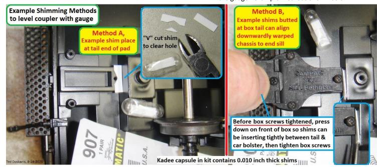
Note: If coupler alignment with gauge is too high, the box may need to be shimmed under its front or overall entirety.
