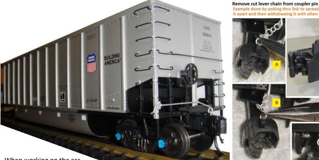
When working on the car with it placed upside-down, it's behooving to first remove its coal load so it won't roll over
