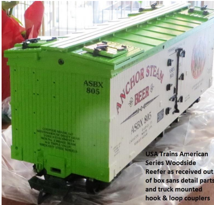
Woodside Reefer now with body mounted 3-D printed CamPac Box™ fitted with Kadee center set coupler in factory draft gear opening - albeit modified
