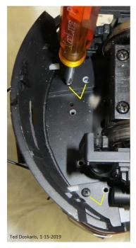
Remove pilot to chassis fasteners (2 possible screws each side) then lift out pilot from chassis crevasse
