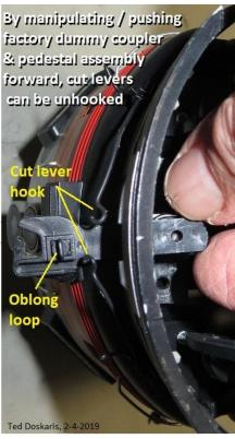
Note: If equipped with factory dummy coupler assembly, unfasten the pedestal and the pilot (described next), and then carefully withdraw all together. This would also make it easier should cut levers that are festooned to the "knock-out" plug be difficult to unhook. Withdrawing the dummy coupler and removing the knock-out plug from the pilot are later described in step 5.
