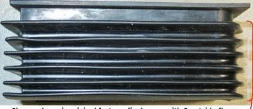
Shown above is original factory diaphragm with 6 outside flues — Shown below is modified diaphragm - reduced to 3 outside flutes
