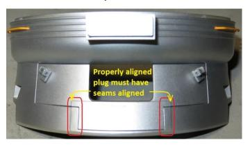
USA Trains F3A Pilot Knock-out Plug Removal Method (Installation in reverse order from shown)
