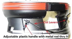
Rod could be withdrawn from pilot & plastic handle
