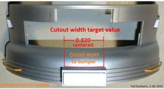
Removed plug facilitates use of machinist scale.
