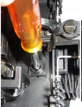
Remove factory (or aftermarket) coupler with pedestal from rear of F3 A unit - both ends of B unit.
