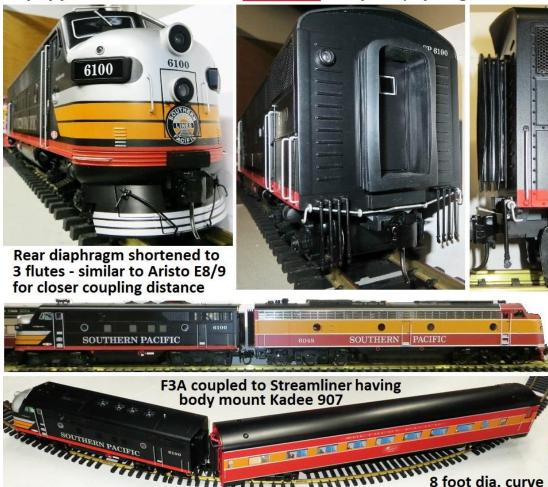
Installing 3-D Printed pedestal and coupler box components on F3A & B units
