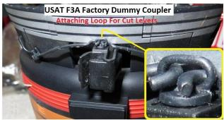
Dummy coupler turned 90°, then wiggled whilst pulling thru
