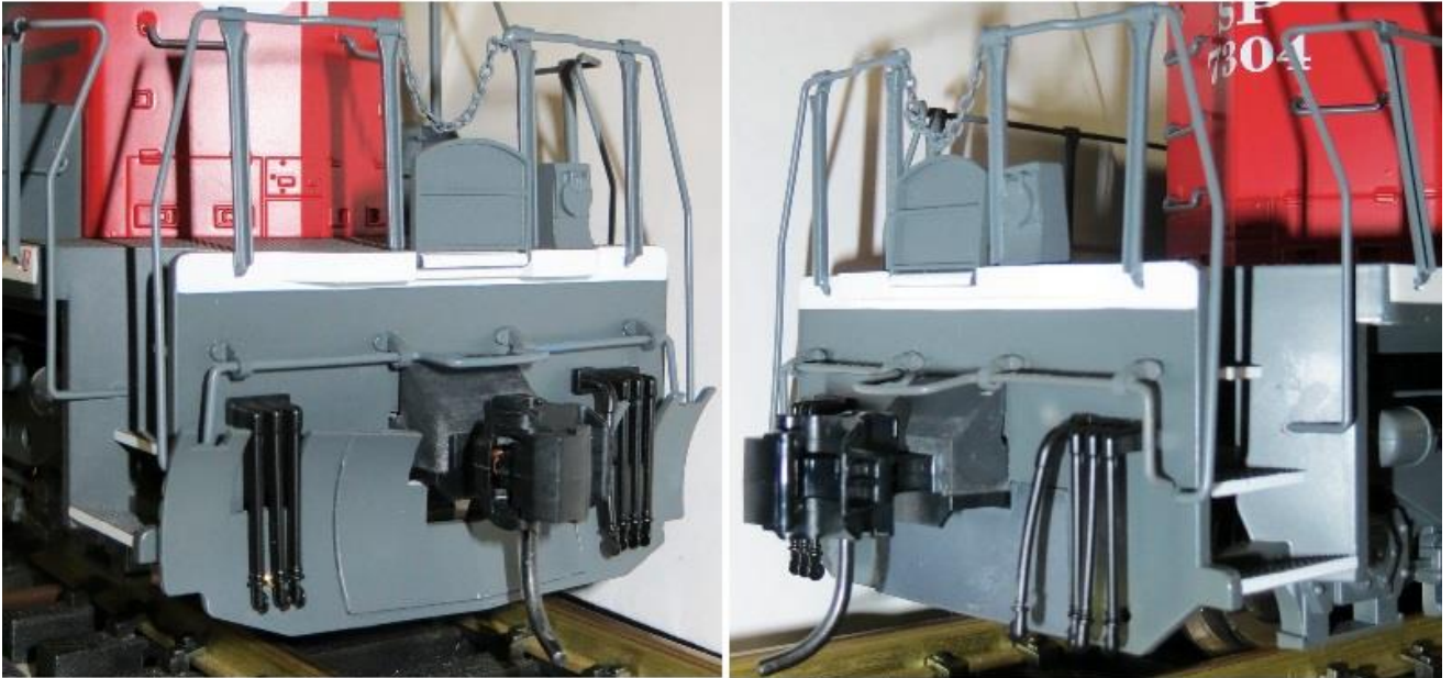
Completed installation, SD40-2 front & rear CamPac Box with integrated fairing
