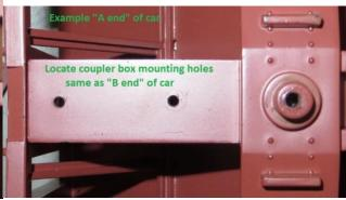
The CamPac Box<sub>TM</sub> can be used as template to locate holes. Mounted Box may need shim:
