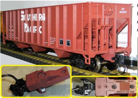
Car "B end" identified by brake wheel. Note that trucks are to have factory coupler tang removed for rotational clearance.
