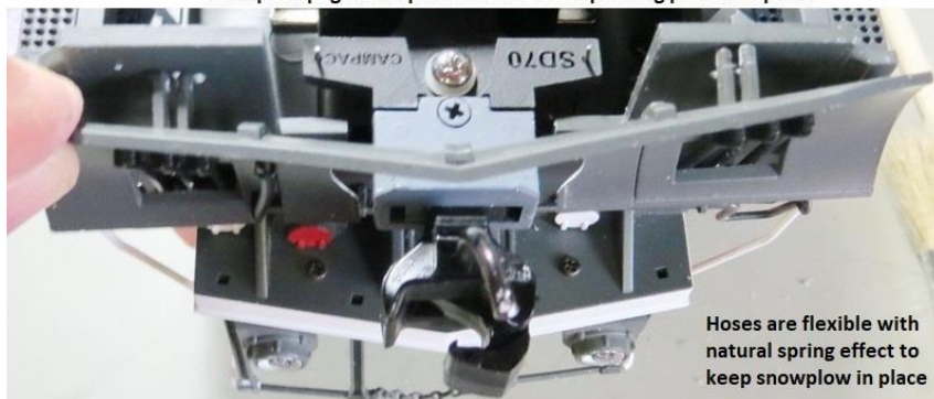
Snowplow pegs to be press fit into corresponding pilot hole pairs:
