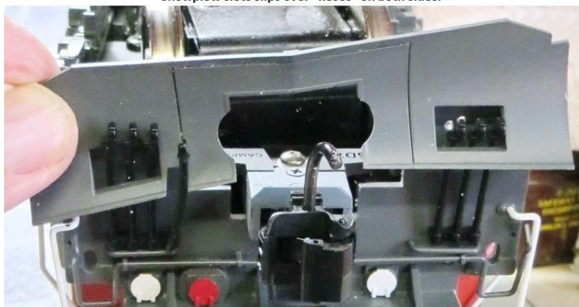
Snowplow pegs to be press fit into corresponding pilot hole pairs:
